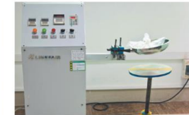
Arm Drop Test Machine
