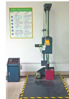
Arm Drop Test Machine
