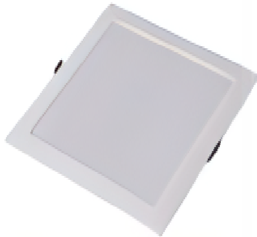
199F/18W MAT:ABS+PS SIZE:180*180MM CUTOUTSIZE:140*140MM 3000K/4000K/6500K
