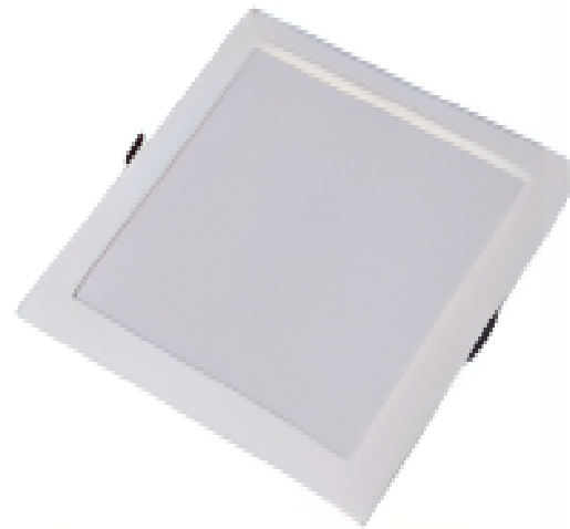
199F/7W MAT:ABS+PS SIZE:120*120MM CUT OUT SIZE:95*95MM 3000K/4000K/6500K
